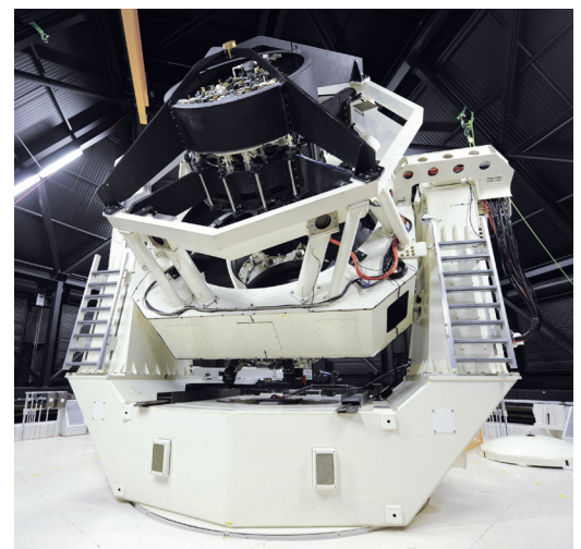
Figure 1. Left, the wide field-of-view CCD in the integration test lab at Lincoln Laboratory. Note the curvature of the image of a fluorescent bulb at the top of the unit. Right, the core of the Space Surveillance Telescope comprising a two-axis mount, large horizontally rotated yoke, and Mersenne-Schmidt optics in the center. The wide field-of-view CCD is located at the base of the central column.
