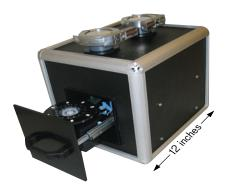
For aerosol samples, the 37 lb, 1 ft<sup>3</sup>, portable PANTHER sensor called CUB (for Compact Unit Biosensor) has shown identification of pathogens in a record time of <2 minutes, and its modest cost, less than \$30,000, makes it viable for widespread biodefense use.
