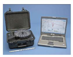
For liquid samples, the Laboratory developed a 16-channel sensor that processes ~100 samples in an hour. This unit has higher throughput than that of any competing technology.
