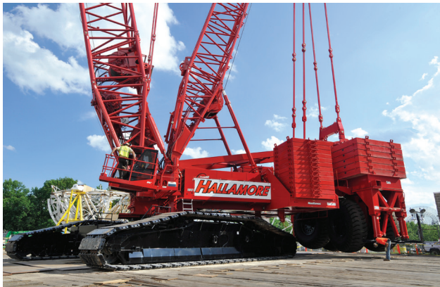
FIGURE 16. Under heavy loads, the crane's 230-ton auxiliary counterweight lifts completely off the ground.
