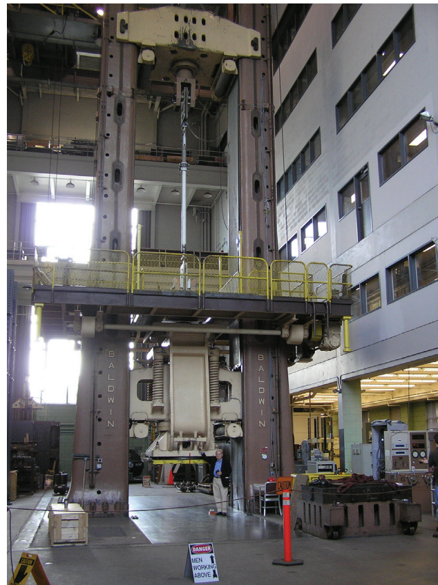
FIGURE 30. The 12-foot-long reflector support struts were tested to more than 200% of the design load in both tension and compression in Lehigh University's testing machine (note the person on floor for scale).
