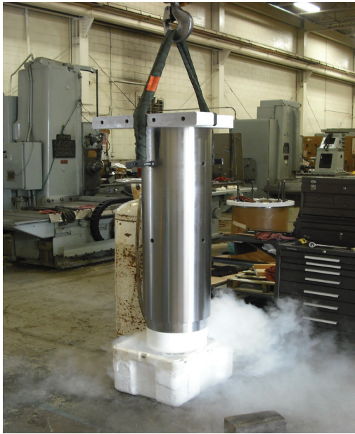
FIGURE 22. Liquid nitrogen boils as the 6-foot-long stub shaft is lowered in. Once cooled, the stub shaft is pressed into the inner race for a permanent “thermal fit.”
