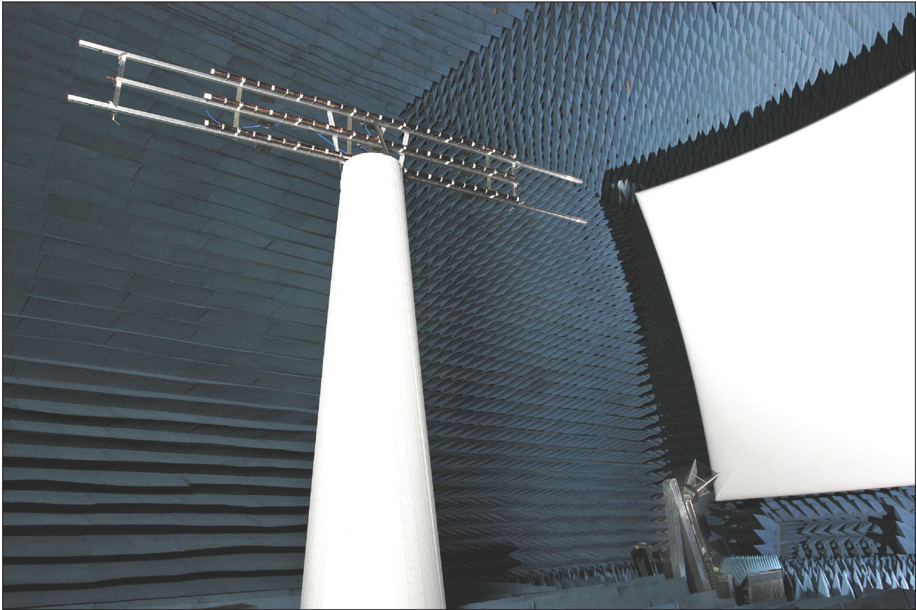
FIGURE 8. Large UHF array under test in the new compact range chamber. The array is shown mounted on a large foam tower that reduces electromagnetic scattering effects. A lower-azimuth positioner (not shown) provides the desired antenna rotation.
