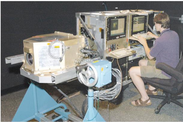
**FIGURE 1.** Jigsaw ladar, data acquisition computer, Global Positioning System (GPS), inertial navigation unit (INU), and operator.
