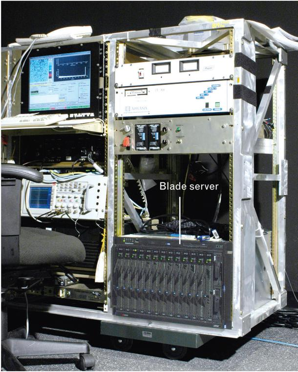
**FIGURE 19.** IBM Blade server cluster installed at bottom of the Jigsaw computer rack.
