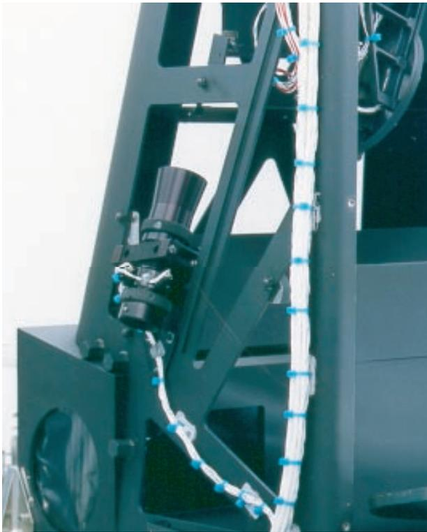
**FIGURE 17.** Photograph of internal reference source mounted on the ALI frame.
