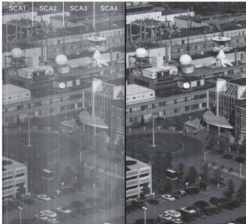
**FIGURE 13.** Band 3 image of Lincoln Laboratory. The image on the left is prior to radiometric calibration. The image on the right is after radiometric calibration.
