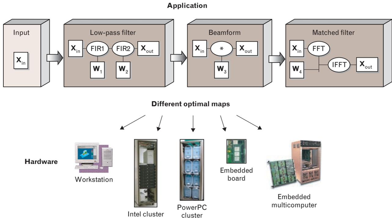
**FIGURE 16.** Optimal mapping challenge. Real applications can easily involve several complicated processing stages with potentially thousands of mapped vectors, matrices, and computations. The maps that produce the best performance will change, depending on the hardware. Automated capabilities are necessary to generate maps and to determine which maps are optimal.
