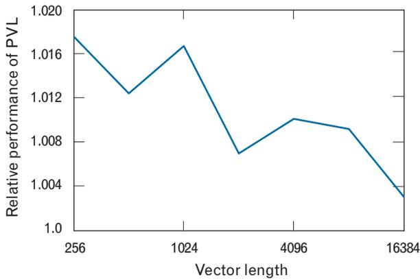
**FIGURE 10.** Overhead for PVL fast Fourier transform (FFT) execution time, relative to that of the Fastest Fourier Transform in the West (FFTW) library for vectors of various lengths. In all cases the overhead is less than 2%.
