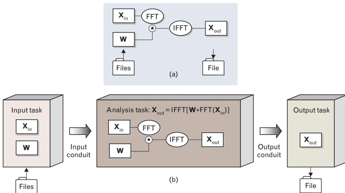
**FIGURE 7.** (a) Development of a basic frequency-domain filtering application, using an FFT and an inverse FFT (IFFT) on input data. PVL vector/matrix and computation objects allow signal processing algorithms to be implemented quickly by using high-level constructs. (b) PVL tasks and conduit objects allow complete filtering systems to be built.
