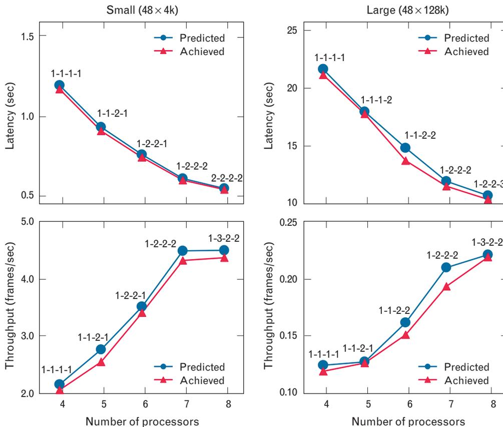
**FIGURE 18.** S3P performance. The S3P framework is tested on two different problem sizes in a four-stage application with two different criteria: minimize latency for a given number of processors and maximize the throughput for a given number of processors. In all cases S3P picks the correct mapping, as shown by the four-component processor assignment string, and predicts the performance of the best map to within a few percent.
