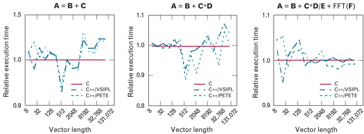
**FIGURE 14.** Comparison of multiprocessor (with communication) performance of VSIBL (C), PVL (C++) on top of VSIBL (C), and PVL (C++) on top of PETE (C++) for three different expressions with different vector lengths. PVL with VSIBL or PETE is comparable to the performance of VSIBL.
