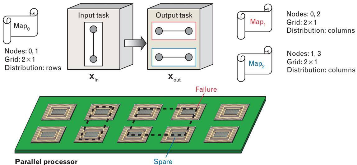
**FIGURE 15.** Dynamic mapping for fault tolerance. The separation of mapping from the algorithm allows the application to adapt more easily to changing hardware by modifying mapping at runtime. Remapping a matrix, for example, allows the program to react to failed processors and assign the work load to a spare processor, without requiring any fundamental change in the signal processing algorithm.
