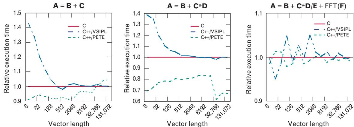
**FIGURE 13.** Comparison of multiprocessor (no communication) performance of VSIBL (C), PVL (C++) on top of VSIBL (C), and PVL (C++) on top of PETE (C++) for three different expressions with different vector lengths. PVL with VSIBL or PETE is comparable to or better than the performance of VSIBL.
