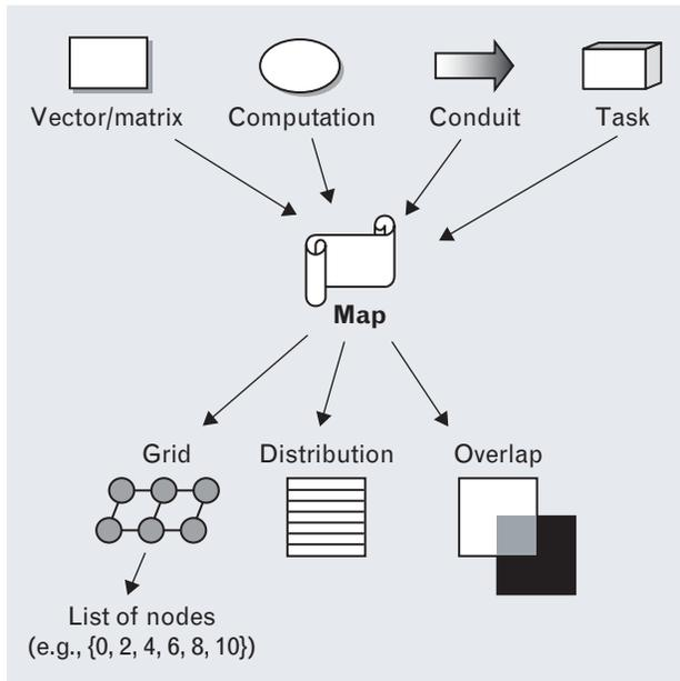
**FIGURE 8.** Structure of a PVL map object. All PVL user objects contain a map. Each map is composed of three components: a grid, a distribution description, and an overlap description. Within the grid is the list of physical nodes onto which the PVL object is mapped.
