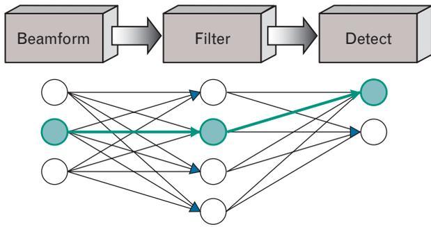
**FIGURE 17.** Self-optimizing Software for Signal Processing (S3P). This framework combines the dynamic mapping capabilities found in PVL with the self-optimizing software techniques developed in FFTW. The resulting framework allows an optimal mapping to be found automatically for any application on any parallel architecture. Each available path is a complete system mapping, and the best path (shown in green) is the optimal system mapping.
