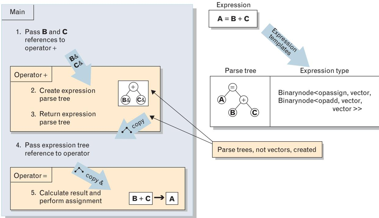
**FIGURE 11.** C++ expression templates. C++ typically requires the use of temporary variables in order to write high-level mathematical expressions. Obtaining high performance from C++ requires technology such as expression templates that eliminate the normal creation of temporary variables in an expression.
