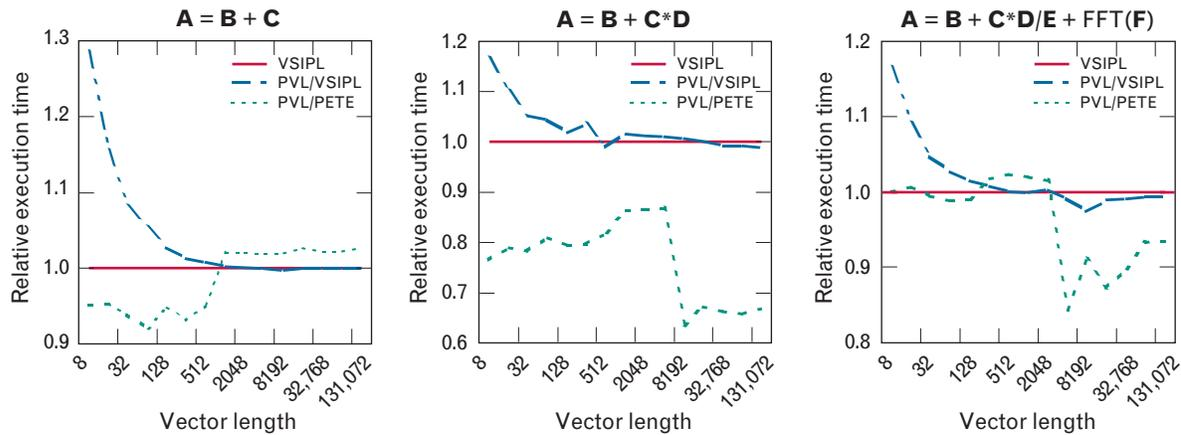
**FIGURE 12.** Comparison of single-processor performance of VSIBL (C), PVL (C++) on top of VSIBL (C), and PVL (C++) on top of the Portable Expression Template Engine (PETE) (C++) for three different expressions with different vector lengths. PVL with VSIBL or PETE is able to equal or improve upon the performance of VSIBL.
