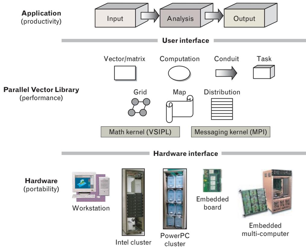
**FIGURE 5.** PVL layered architecture. The main purpose of a software library as middleware is to insulate the application from the hardware. The user writes an application in the high-productivity layer. The middleware implements constructs necessary to deliver high performance on parallel computers. The portability of the middleware is achieved by isolating the hardware-specific details to a math kernel such as VSIP and a messaging kernel such as MPI.
