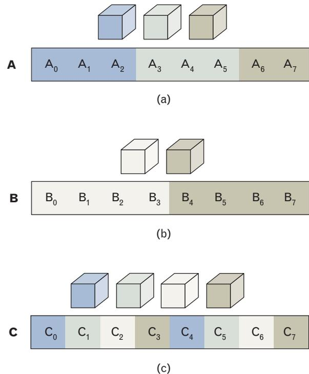
**FIGURE 9.** Example distributions of a vector of length eight: (a) block distribution on three processor nodes, (b) block distribution on two processor nodes, (c) cyclic distribution on four processor nodes.
