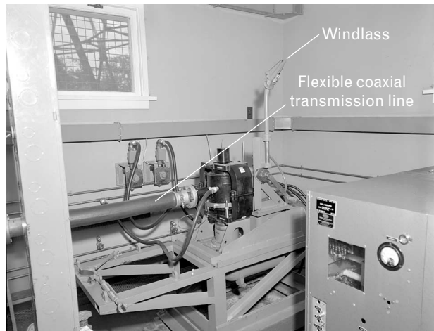
FIGURE 1. Transmitter of the AN/FPS-31 (XD-1) UHF ground control of intercepts (GCI) radar. The QK-508 magnetron (middle) fits into a pulse transformer and is powered by the modulator cabinet on the right. The high-power RF output pulses travel from the magnetron through a section of 3-1/8-in flexible coaxial transmission line (at the left) to the vertical waveguide run (see also Figures 2 and 3). Note the windlass (essential when changing magnetrons) and the arrangements for liquid cooling of the magnetron.
