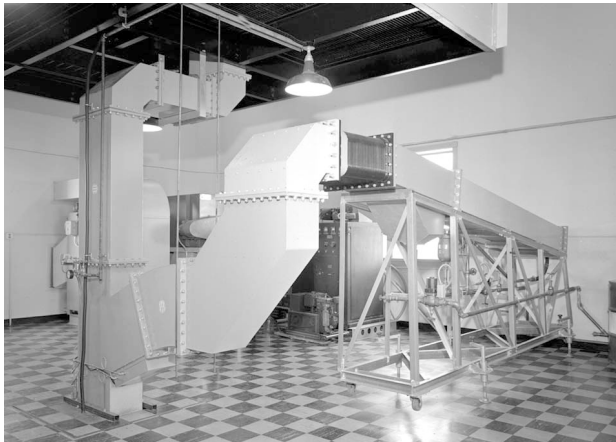
FIGURE 10. Dummy RF load for the transmitter of the UHF GCI/CCM radar. The transmitter is on the floor below; the rotary joint and antenna mount are on the floor above. A waveguide switch allows for operating with the dummy load (right) or the antenna (upstairs). For scale reference, each floor tile measures 9 \times 9 in.
