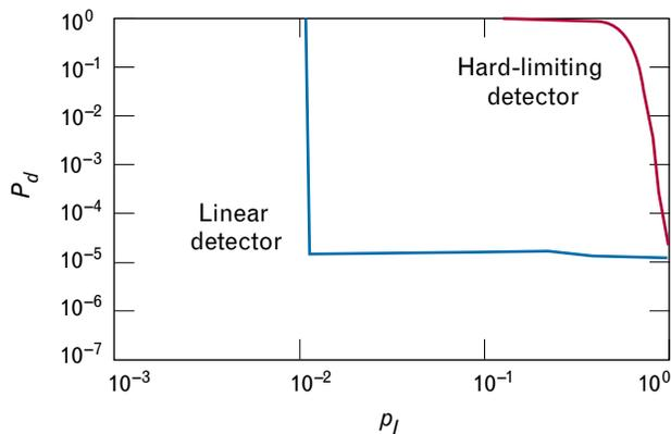
**FIGURE 5.** Probability of detection  $P_d$  at the output of a digital integrator versus the probability of interference  $p_I$ . Interference was 100 times noise. Peak signal amplitude was the square root of 10 times the wideband noise variance.
