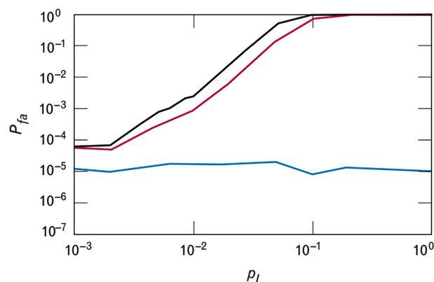
**FIGURE 4.** Probability of false alarm  $P_{fa}$  versus probability of interference  $p_I$ . The black curve represents data from a linear receiver with interference 100 times the noise. The red curve represents data from a linear receiver with interference 10 times the noise. The blue curve represents data from a hard-limiting receiver with interference 10 times the noise. Only the hard-limiting receiver maintains a  $P_{fa}$  value of  $10^{-5}$  for all values of  $p_I$ .
