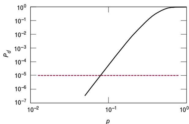
**FIGURE 2.** Probability of detection  $P_d$  at the output of a digital integrator versus the probability  $p$  of a threshold crossing on a single trial. The sliding window is sixteen units long. Eight or more threshold crossings constitute a detection. A useful detection probability of 0.9 can be attained with those values when  $p$  equals 0.625 or greater.
