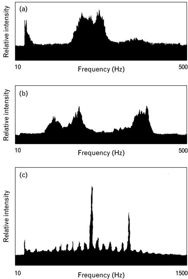
**FIGURE 3.** (a) Doppler spectrum of rainstorm echoes observed with an S-band radar. (b) Doppler spectrum of chaff echoes observed with an S-band radar. (c) Doppler spectrum of a C-45 aircraft inbound observed with an S-band radar.
