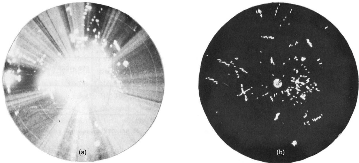
**FIGURE 6.** Comparison of displays from two receivers subjected to three jammers on a single B-47 at 35,000-ft altitude and 10-mi range: (a) time exposure of an output display of a linear receiver and (b) time exposure of the output of a hard-limiting receiver. The lines of blips represent aircraft tracks.
