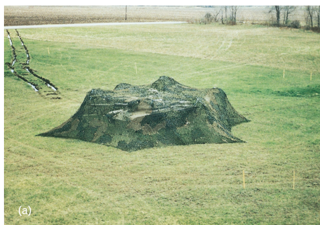
FIGURE 16. (a) Visible-light photograph and (b) GaAs (0.85 \mu\text{m} ) laser-radar angle-angle-range image of a tank concealed by a camouflage net. The laser radar utilizes a high-accuracy, sinusoidal, amplitude-modulated waveform while observing the tank in a downlooking scenario. The camouflage net was readily gated out of the image to leave the tank image. The tracks left by the tank in the soil are also visible in the laser-radar image.
