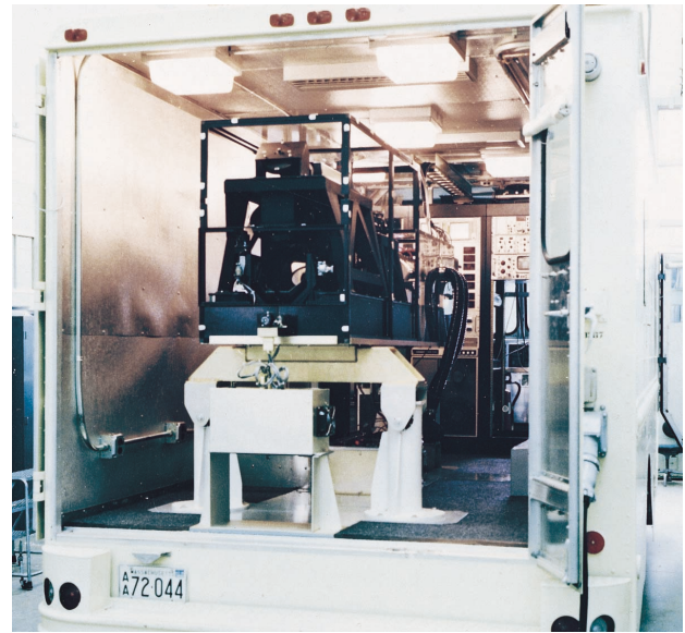
FIGURE 9. Transportable multisensor measurement system consisting of a coherent CO 2 laser radar with a boresighted and pixel-registered 8-to-12- \mu m passive infrared sensor and digital recording system.
