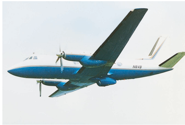
FIGURE 12. Gulfstream G-1 aircraft with the Infrared Airborne Radar (IRAR) optical aperture located in the ventral fairing on the aircraft. The IRAR test bed carried a wide variety of active and passive sensors over a ten-year period.
