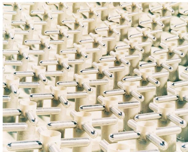
**FIGURE 12.** The FSS used for the U.S. Army SAFEGUARD System Command propagation study, comprising an array of L-band crossed-dipole elements mounted on a low-loss, plastic, hyperboloidal substrate. The loss in antenna gain at L-band was less than 0.2 dB and was negligible at UHF.
