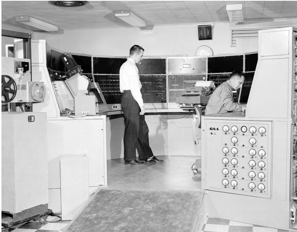
**FIGURE 4.** Original Millstone site CG-24 computer, circa 1960. All functions performed by the CG-24, which took up an entire room, could now be performed by one of today's desktop computers.
