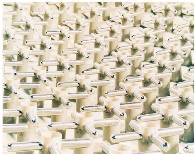
**FIGURE 12.** The FSS used for the U.S. Army SAFEGUARD System Command propagation study, comprising an array of L-band crossed-dipole elements mounted on a low-loss, plastic, hyperboloidal substrate. The loss in antenna gain at L-band was less than 0.2 dB and was negligible at UHF.
