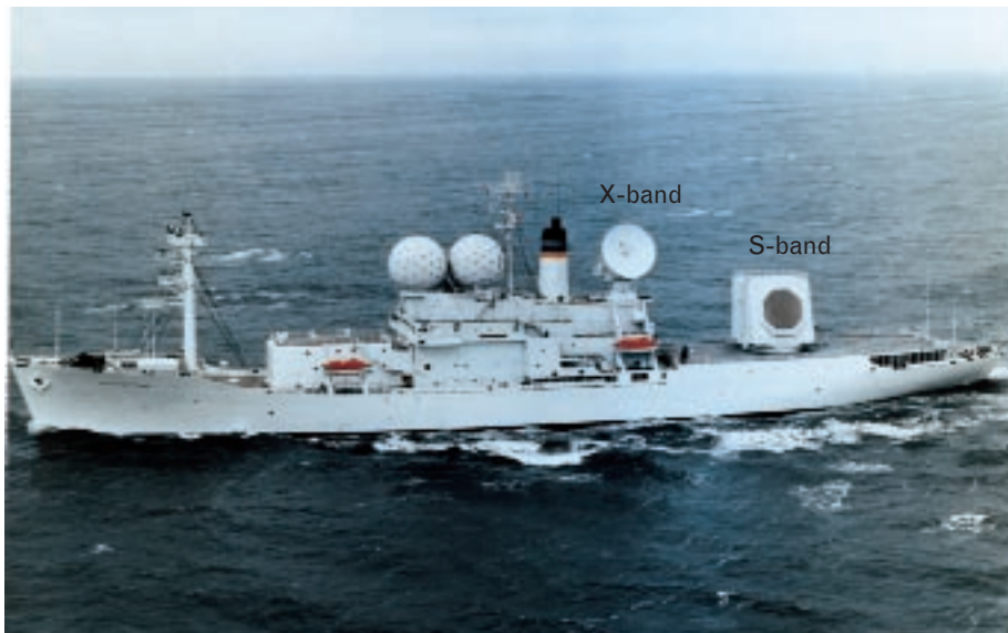
FIGURE 4. The COBRA JUDY ship with a clear view of the S-band phased-array and X-band dish-antenna radars.
