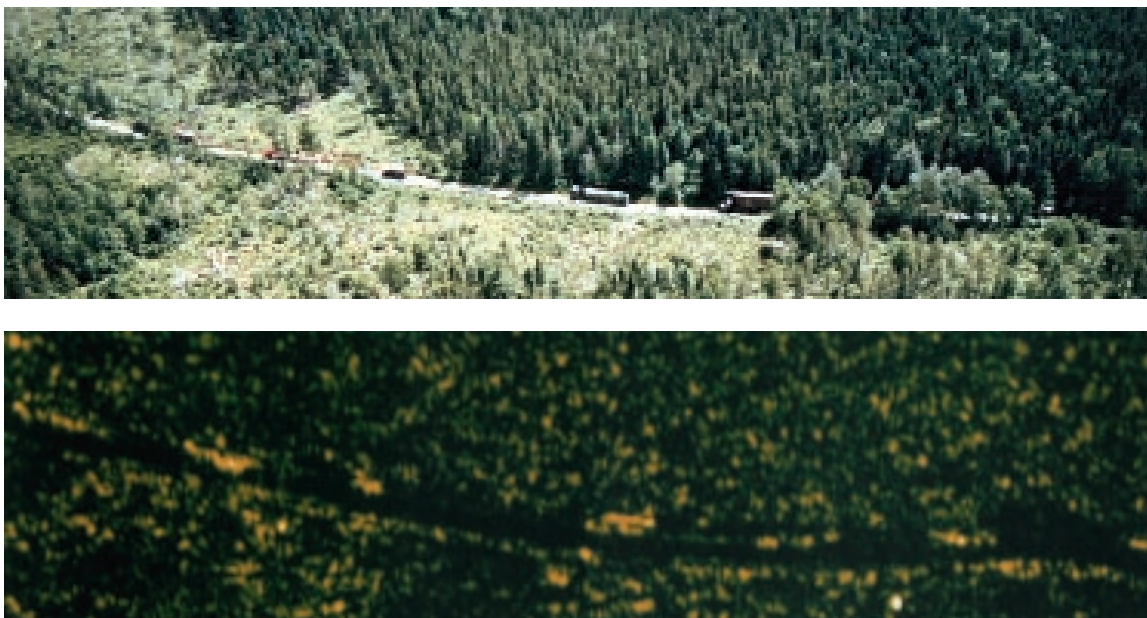
FIGURE 12. Aerial photo (top) and SAR image (bottom) of the Cedar Swamp, Maine, deployment. The radar line of flight in the SAR image was across the top of the photo. The vehicles in the center were not visible from the point of view of the radar because of the thick foliage.
