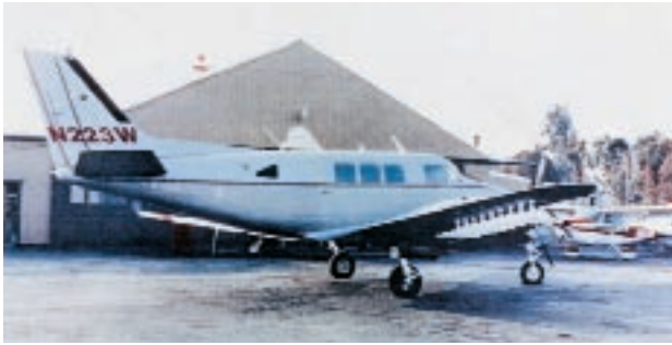
FIGURE 11. SRI International ultra-wideband UHF SAR. The antenna is mounted under the wing of the aircraft. The SAR parameters are listed in Table 1.
