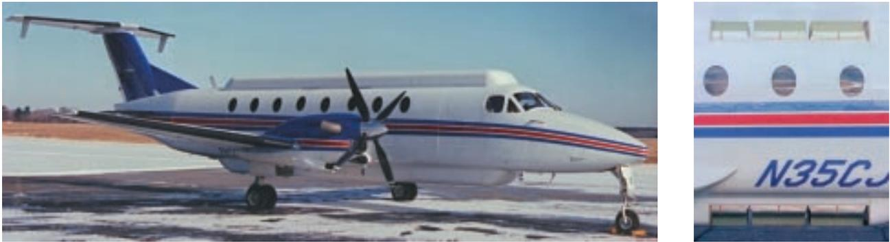
**FIGURE 6.** Beechcraft 1900 aircraft (left) configured for the technology demonstration. An array of eleven antenna elements is mounted under radomes along the top and bottom of the fuselage in pairs that act as dipoles. The inset (right) shows the antenna elements without radomes.
