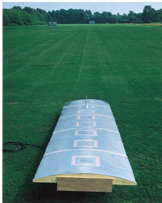
FIGURE 3. TCAS antenna measurements at the Lincoln Laboratory Antenna Test Range (ATR). In the foreground, the TCAS antenna and VHF blade antenna are mounted on a mock-up of a Boeing 727 fuselage. During the experiments, the fuselage was mounted in an anechoic chamber (Figure 4). At the far end of the range is the dish antenna that provides the signal source used for the bearing-error measurements.
