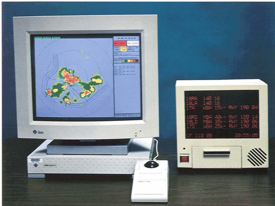
FIGURE 2. In the TDWR system, the Situation Display (SD), shown in the left, and the Ribbon Display Terminal (RDT), shown in the right, provide key information to air traffic users. The SD shows the locations of wind-shear events on a precipitation reflectivity background, and the RDT provides alphanumeric wind-shear alert messages in a format suitable for direct readout.
