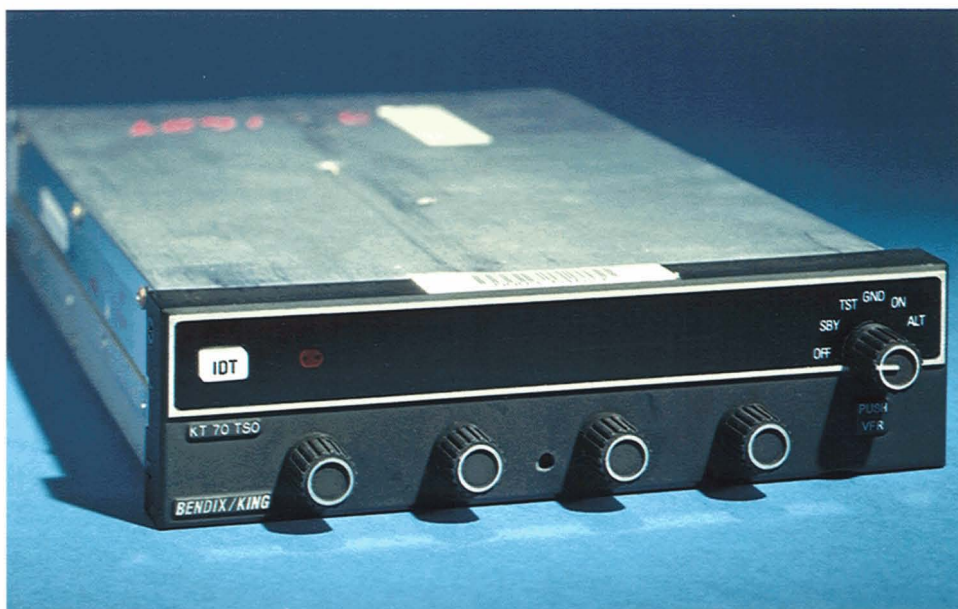
FIGURE 3. Mode S transponders similar to the panel-mount model pictured here, with a retail price of approximately $3000, can provide data-link capability to general aviation (GA) aircraft.
