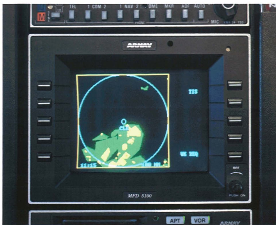
FIGURE 4. Data-link control and display unit (CDU) as installed in the instrument panel of the Cessna 172 data-link test-bed aircraft. Shown is a color radar precipitation image transmitted to the aircraft by Mode S data link. Color LCD technology shows promise for low-cost data-link CDUs in the $2000 to $5000 price range.
