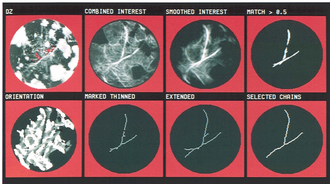
FIGURE 9. Extraction steps. Candidate gust fronts are extracted from a combined interest image. For a description of the different steps involved, see the subsection "Extraction" in the main text.
