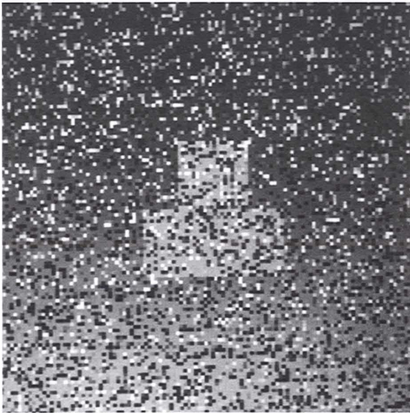
FIGURE 3. The image of Figure 2 has been synthesized for a carrier-to-noise ratio (CNR) of 10 dB, corresponding to an image in which 20% of the pixel values are anomalous. (An anomaly is defined as a pixel value in the corrupted image that differs from the value in the original image by more than two range counts.) Each pixel in the image has 8 bits (256 gray levels) of resolution.
