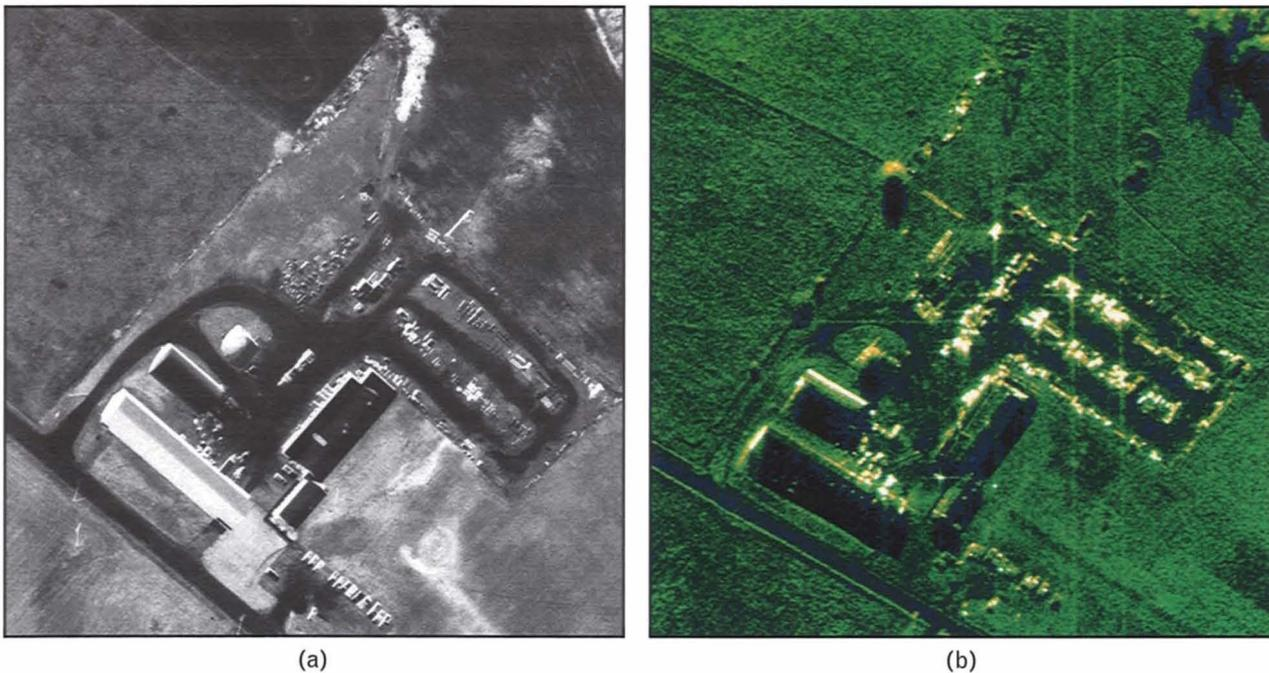
**FIGURE 14.** (a) An optical photograph and (b) a SAR image of a farm-supply store in Stockbridge, New York. This store is an example of a man-made clutter discrete. The store parking lot is in the bottom of each image. Although the photograph and the SAR image were taken at different times, passenger cars can be seen in the parking lot in both images. The bright spots in the middle right area of the SAR image are caused by various metallic objects in the yard of the supply store.
