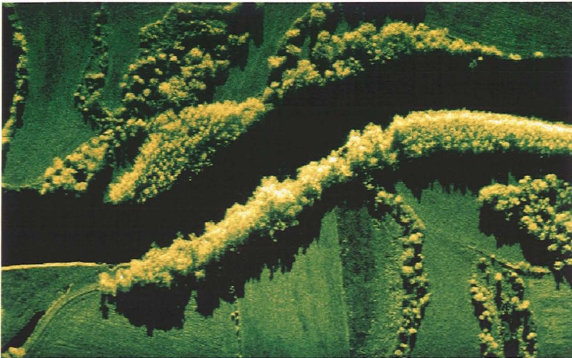
**FIGURE 13.** SAR image of natural clutter in Stockbridge, New York. The sensor is flying parallel to the top of the image, and the shadows extend downward in the image. Areas of high radar return are colored in bright yellow; areas of low radar return are in dark colors. The dark band in the middle of the image is a river with trees lining each bank. The smooth green areas are open fields.
