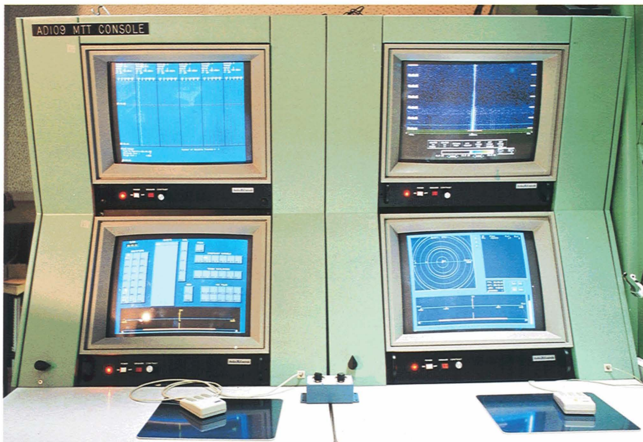
FIGURE 8. The MTT operator's console. The range-time-intensity (RTI) display and the metric display, on the right side of the console, show the locations of the targets to the MTT metric analyst. The signature display and the control-panel display, on the left side of the console, show the radar cross section of each target and allow the signature analyst to identify individual targets and provide MTT state vectors for the TRADEX L-band data-recording system.
