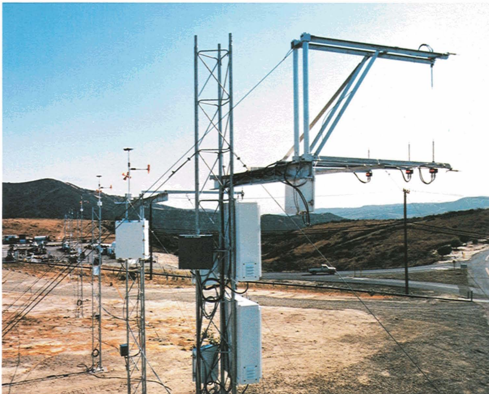
FIGURE 7. Meteorological instruments on towers. This photograph was taken during preliminary measurements of atmospheric characteristics along the 400-m beam path. For the actual propagation experiments, the towers were much more densely spaced. The beam was propagated to the right (upwind) of the towers at the level of the instruments. For the 400-m tests, the receiver trailer sat on the knoll in the distance.
