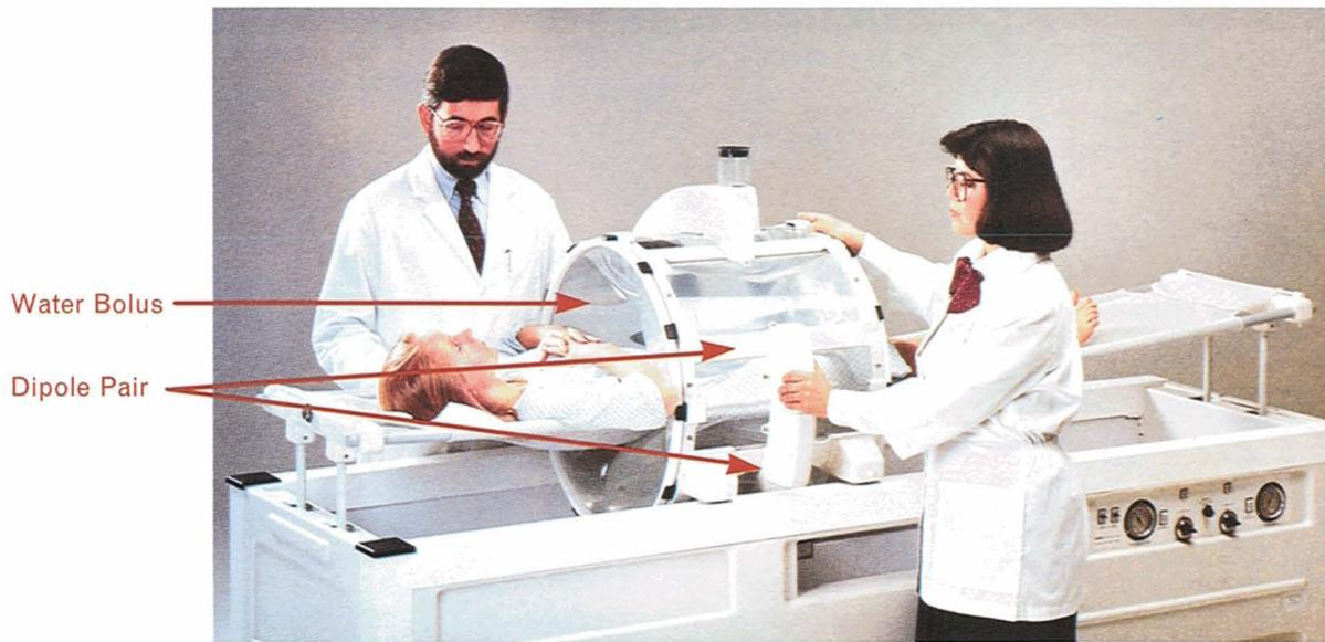
**FIGURE 1.** BSD-2000 hyperthermia system. The 59-cm-diameter annular antenna consists of eight dipoles that are fed as four active pairs of elements. The system operates over the frequency band from 60 to 120 MHz with up to 500 W average power per channel. A cool water ( $5^{\circ}$  to  $40^{\circ}\text{C}$ ) bolus between the patient and the annular array prevents excess heating of the skin surface.
