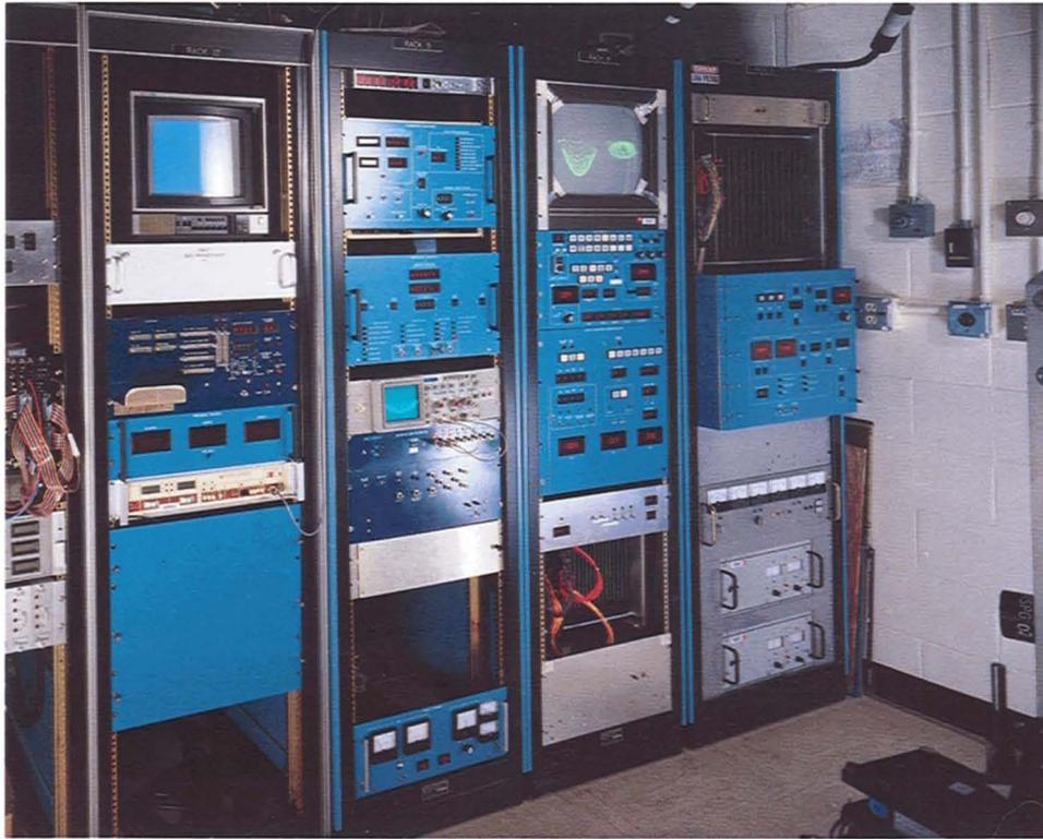
**FIGURE 4.** SWAT control electronics for adaptive optics. From right to left, the racks contain (1) driver electronics for the deformable mirror, (2) a wavefront reconstructor (bottom) and a real-time display for wavefront-sensor data (top), (3) electronics for data formatting and overall system control, and (4) a video display for the charge-coupled device (CCD) far-field camera.
