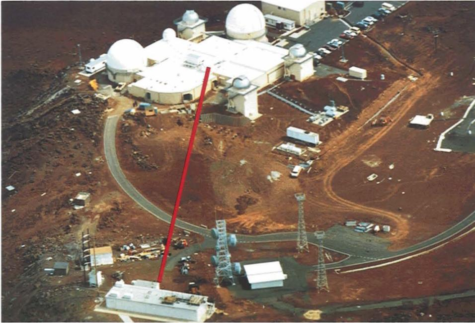
**FIGURE 10.** Site of the horizontal-path measurements at AMOS. The red line indicates the 146-m propagation path from the small dome that houses the laser beam director to the instrumented target trailer.
