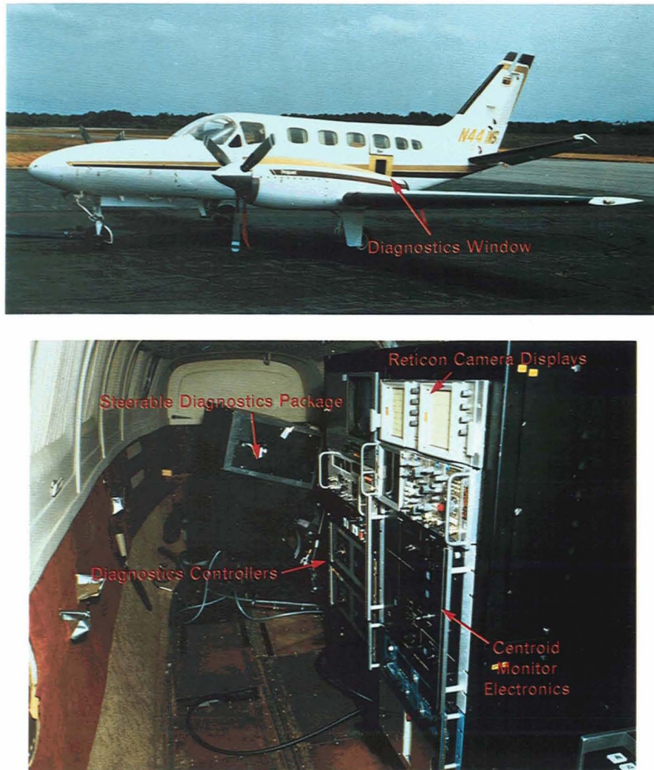
FIGURE 11. Diagnostic aircraft for ACE experiments (1983). The Phase II ACE experiments used this Cessna 441 Conquest to carry a beacon and diagnostic cameras. During the experiments the aircraft flew in a wide-banked turn 10,000 ft above the site, and a compensated laser beam was aimed through a window in a specially modified door of the aircraft.
