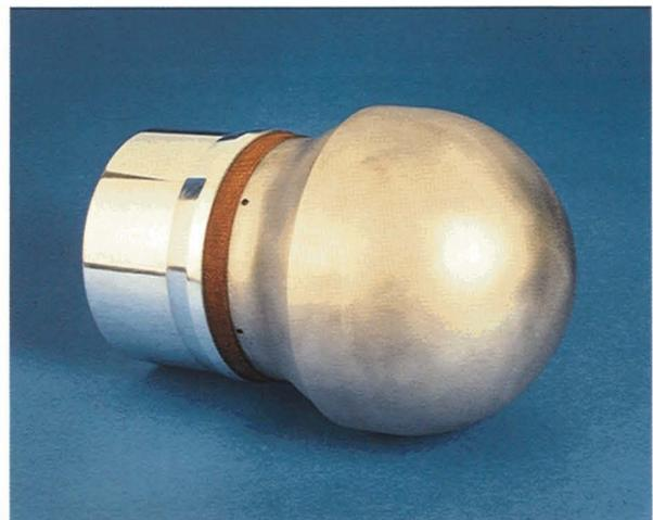
**FIGURE 11.** Later Trailblazer I reentry-body configuration with the annular transmitter housing and antenna mounted aft of the spherical motor, surrounding the motor nozzle. Deleting the transmitter from the original configuration in front of the spherical reentry body placed the body directly in contact with the shock wave.
