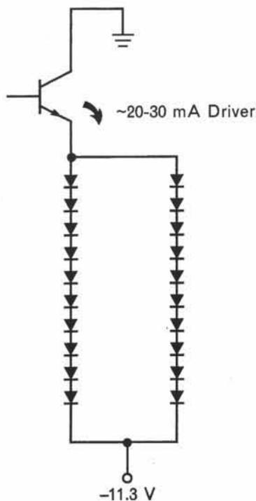
**FIGURE 7.** Fan-out can be achieved with no optical-splitting loss if the lasers are connected in series and parallel. Fan-outs of 20 should be possible with a modest drive current and 1-to-3-GHz operation. The schematic diagram assumes a laser series resistance  $\leq 10 \Omega$ , threshold current  $\sim 5$  mA, and wavelength  $\sim 1.3 \mu\text{m}$ .
