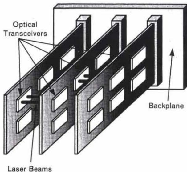
**FIGURE 5.** Free-space optical interconnections allow interconnections to be made in the third dimension in direct paths perpendicular (or at angles) to the boards.
