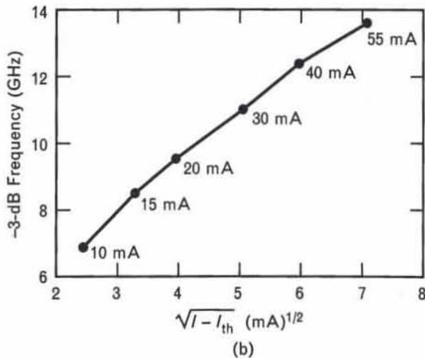
**FIGURE 4.** Performance of 1.3- $\mu\text{m}$  mass-transported buried-heterostructure laser. (a) Output power versus laser current before and after high-reflectivity coating. Note that the coating improves the differential quantum efficiency to greater than 60%. (b) The -3-dB frequency for the laser of part a is more than 12 GHz with only 40 mA of current.
