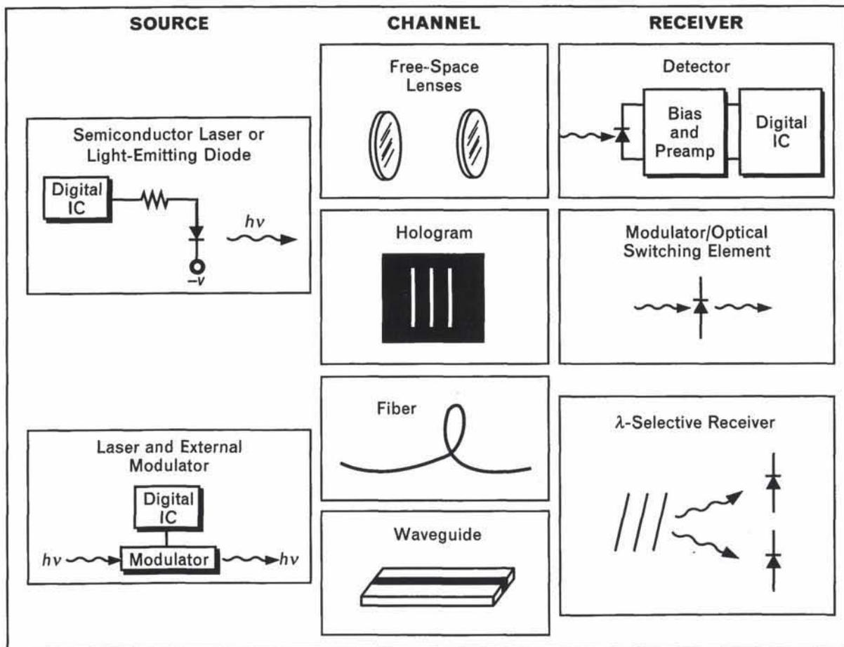
**FIGURE 1.** Optical interconnections can be partitioned into a source, a channel, and a receiver. Some of the various possibilities are shown.
