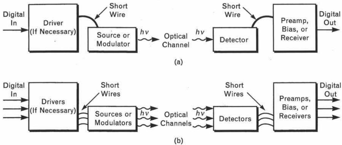
**FIGURE 2.** Optical interconnection systems: (a) single channel and (b) multiple channel. With optical interconnection systems, high-speed interconnections can be made with short electrical lines while the optical link maintains the integrity of the signal. When multiple channels are considered, signal channels can cross one another, optical imaging techniques can be applied, and holographic and reconfigurable holographic channels can be considered.
