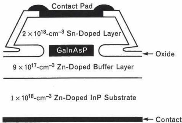
**FIGURE 3.** Cross section of p-substrate mass-transported laser. The contact pad is confined to the top of the laser mesa to minimize parasitic capacitance.
