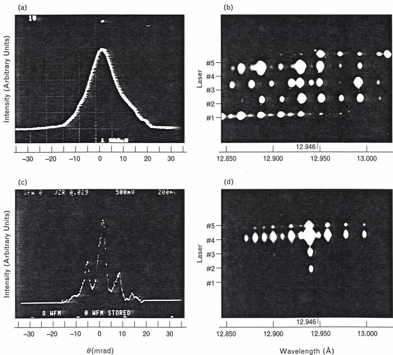
**FIGURE 6.** Far-field pattern (left) and emission spectra (right) of the linear laser array before (upper) and after (lower) the coherent phase locking. The locking is clearly demonstrated by the narrower peaks in the far-field pattern in (c) and by the identical emission spectra in (d).
