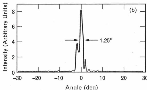
**FIGURE 10.** A monolithic lens laser: (a) the characteristic light output versus drive current, and (b) the far-field radiation pattern.
