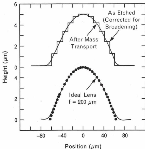
**FIGURE 3.** The profiles of the etched multistep mesa structure and the nearly ideal lens it formed after mass transport.
