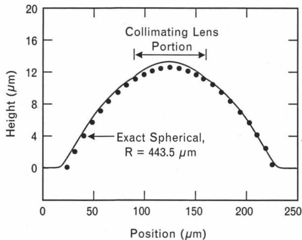
**FIGURE 8.** Bifocal microlens for monolithic integration with a diode laser. The two distinct curvatures shown correspond to the two lens portions.
