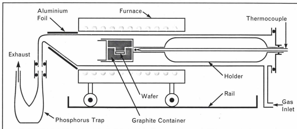
**FIGURE 2.** The furnace system specially designed for mass-transport processing of compound semiconductors. The gas flow, temperature distribution, and furnace movement were designed for high phosphorus vapor pressure along with minimum phosphine consumption and clean phosphorus disposition.
