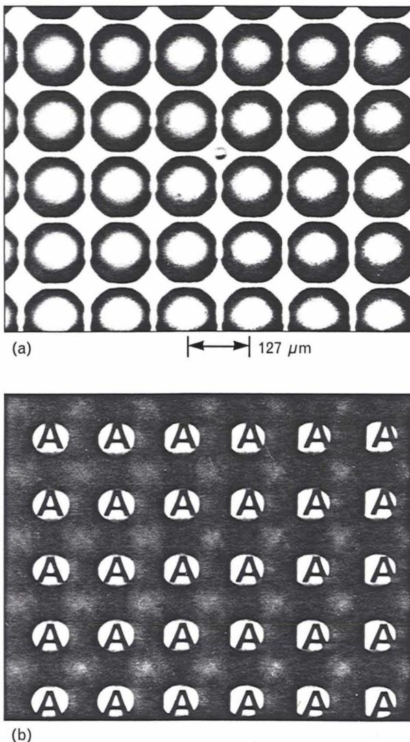
**FIGURE 4.** (a) An array of mass-transported  $f/1$  microlenses in an InP substrate, and (b) the array of images the lens array formed from the letter A placed near the microscope light source.
