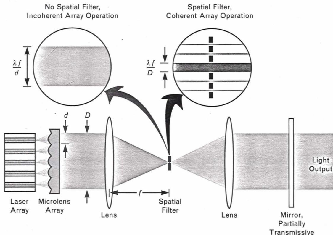
**FIGURE 5.** Coherent phase locking of a laser array in an external cavity. The dimensions in the actual experimental system are  $d = 127 \mu\text{m}$ ,  $D = 635 \mu\text{m}$ ,  $f = 6.25 \text{ cm}$ , and  $\lambda = 1.3 \mu\text{m}$ .
