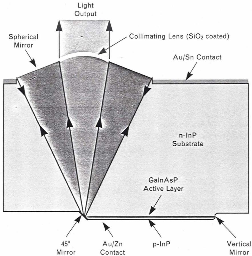
**FIGURE 7.** A diode laser with a monolithic integrated microlens. The longitudinal cross section shows the laser cavity formed by the spherical mirror, the active layer (a buried-heterostructure waveguide gain region), and the vertical mirror at the far end of the waveguide. The central portion of the microlens collimates the laser output.
