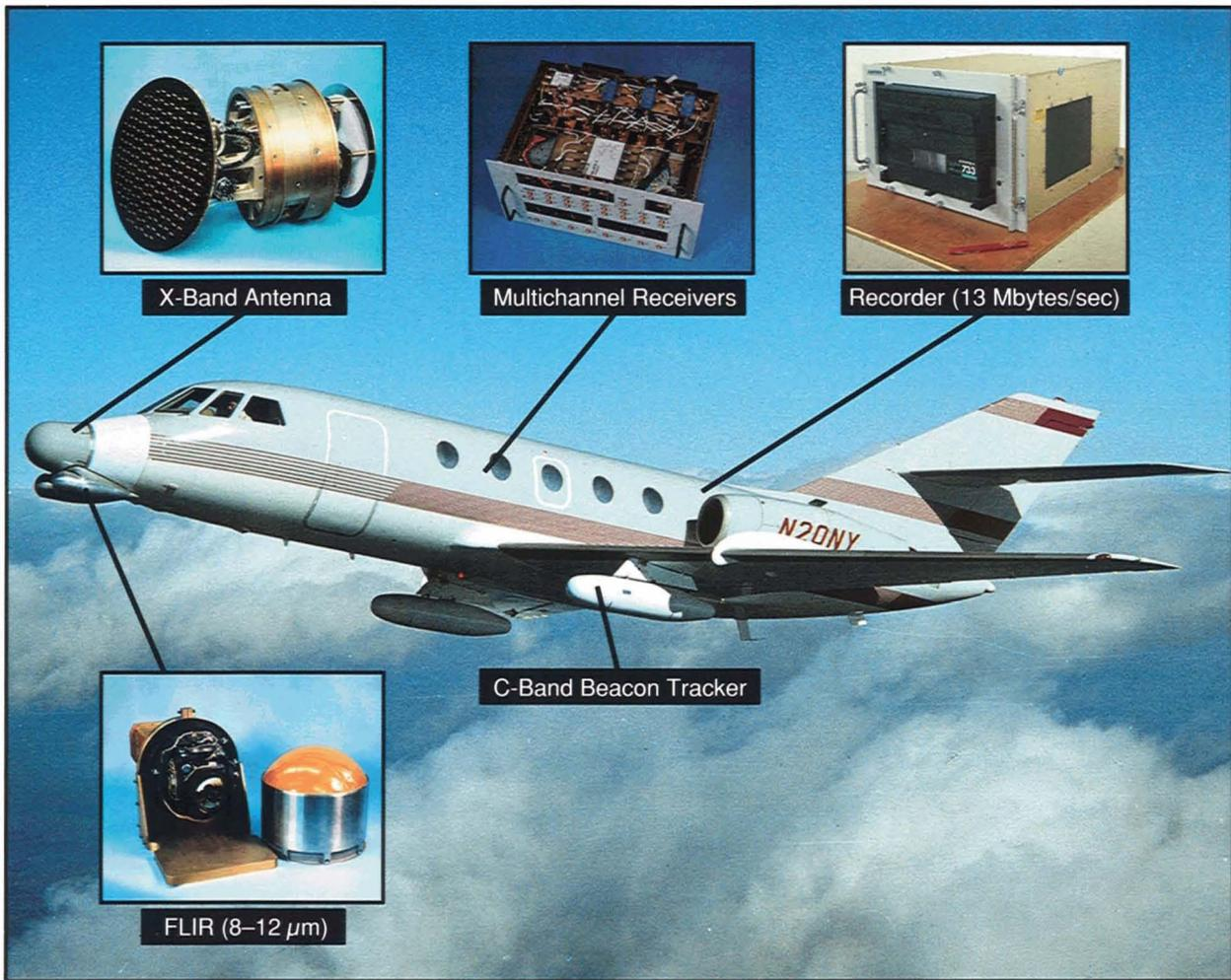
Fig. 3—Principal elements of the Airborne Seeker Test Bed on the Falcon 20 aircraft. The principal sensor, a large X-band dual-polarized monopulse antenna, is supported by a large number of instrumentation channels and a high-speed recorder. A Forward Looking Infrared Sensor (FLIR) provides an angle reference on target position for use with the radar data. A wing-mounted C-band radar locates the target and directs the other sensors.
