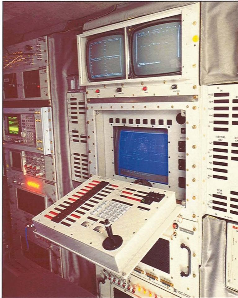
Fig. 11—The operator control panel. The upper-left screen displays received Doppler spectra; the upper-right screen lists target track-file information. The center screen displays system status and the aim point of the gimbaled sensors. The buttons on the lower panel control the stages of an intercept (data recording, sensor acquisition and reacquisition), and initiate mission-specific functions under software control.
