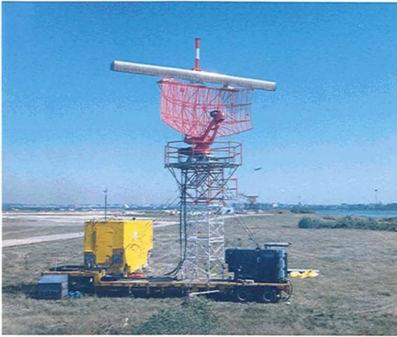
Fig. 15—The Transportable Measurements Facility (TMF) at Washington's National Airport.
