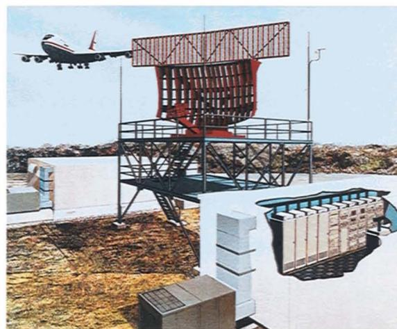
Fig. 17—Mode-S engineering-model sensor.
