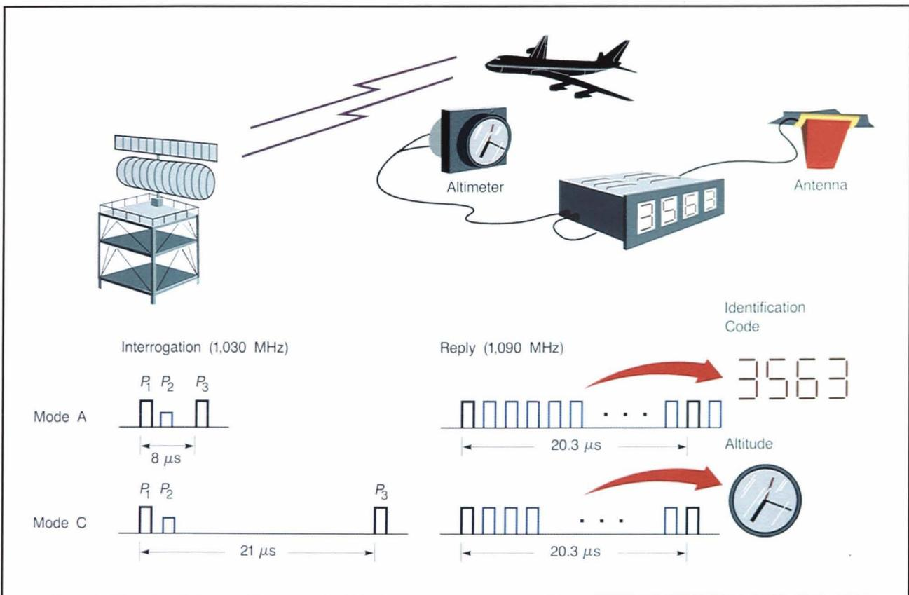
Fig. 1—Air Traffic Control Radar Beacon System (ATCRBS).
