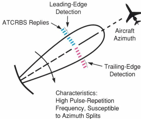
Fig. 4—Sliding-window beam splitter.
