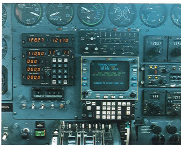
Fig. 14—Mode-S data-link presentation of weather information in the cockpit of a test aircraft.
