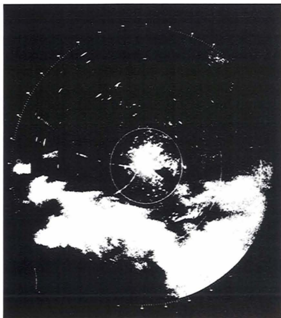
Fig. 8—Comparison of conventional and MTD radar performance in heavy rain. The conventional video image is on the left, and the MTD radar tracker output is on the right.
