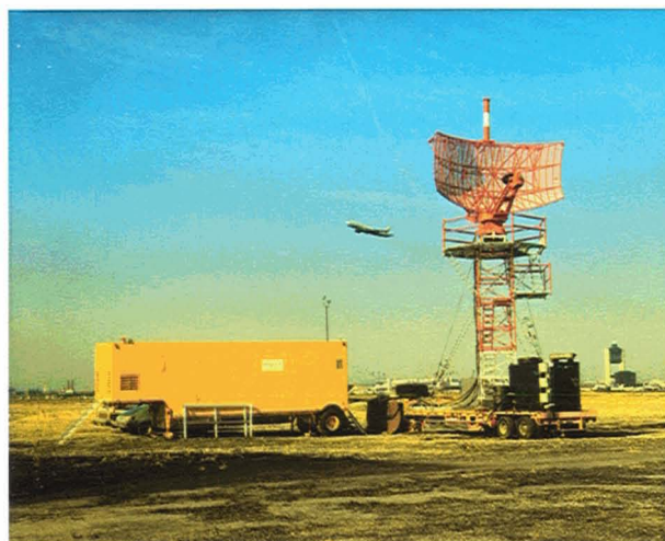
Fig. 3—Early testing of DABS/Mode S, using the Transportable Measurement Facility (TMF) at Logan Airport, Boston.
