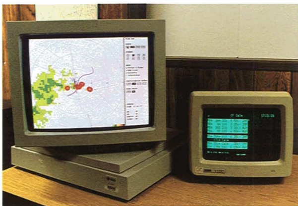
Fig. 10—Graphic and alphanumeric displays of microburst winds detected by an experimental TDWR.
