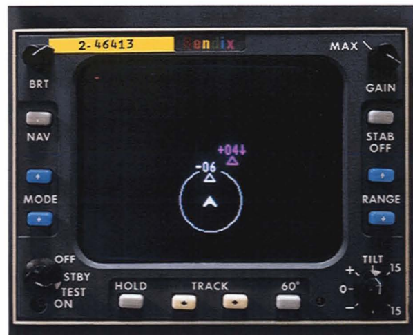
Fig. 12—A TCAS display of conflicting traffic, using modified digital weather radar. The display shows level traffic 600 ft below our own aircraft and ahead at a range of 1.5 mi, along with an aircraft 400 ft above and descending 3 mi ahead at 1 o'clock.
