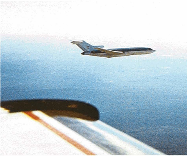
Fig. 13—TCAS testing. This photo was taken from the cockpit of a Lincoln Laboratory test aircraft during controlled encounters with a FAA Boeing 727 aircraft.
