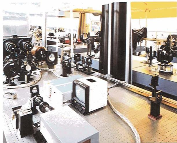
Fig. 10 — (b) Photograph of the adaptive-optics system.
