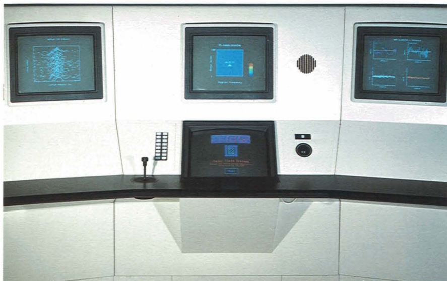
Fig. 5 — The KDS control console includes three high-resolution color screens for real-time information display, a touch screen for operator control, and devices that move on-screen cursors.
