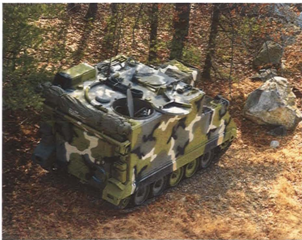
Fig. 28 — Lincoln Laboratory's advanced-development model of the Army SCOTT for EHF satellite communications was installed in an armored personnel carrier and was operated in the field against a satellite simulator by GI crews.
