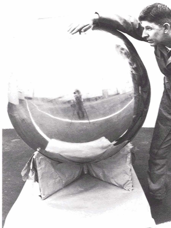
Fig. 16 — A Lincoln Calibration Sphere at Rohr's plant in Chula Vista, Calif. Note in the mirrorlike surface of this sphere the reflection of the man leaning on it, the camera and tripod, the photographer, lines in the parking lot, and surrounding buildings. The man is believed to have been an employee of Rohr; he has not been identified.
