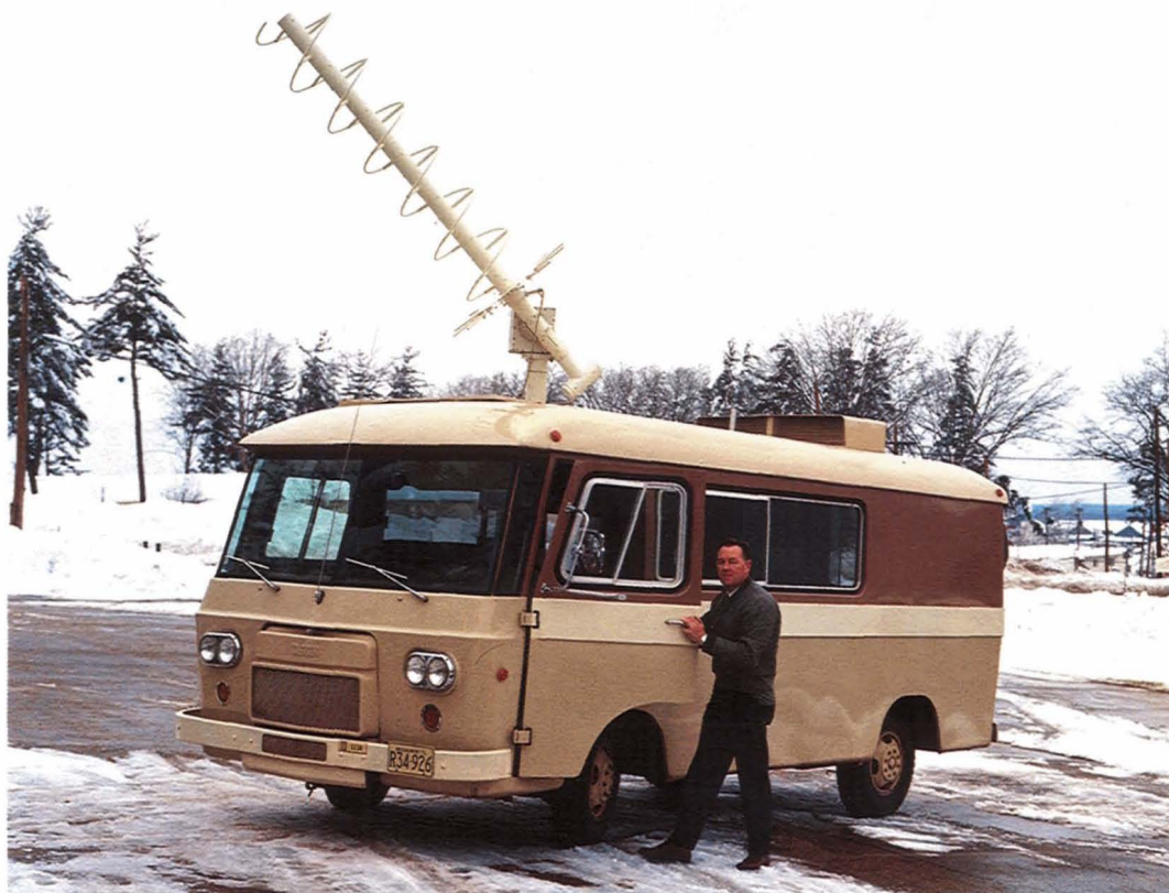
Fig. 14 — Lou Hollowell is about to take off with LET-4, a mobile terminal for UHF satellite communications.
