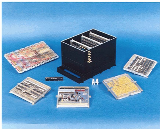
Fig. 7 — Implementation of FEP. The device includes seven boards, weighs 6 lb, and draws 6 W. It includes a real-time emulator, real-time Pascal, and 64K of memory.
