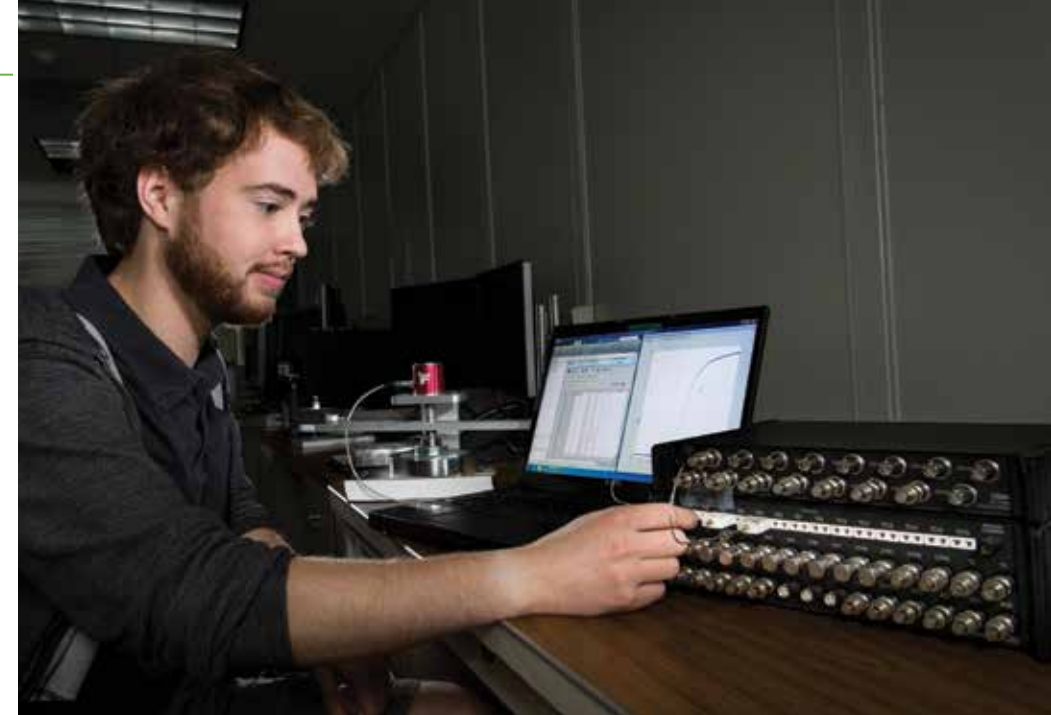
Finn O'Brien, intern from Worcester Polytechnic Institute, sets up the test platform that will be used to determine the thrust of small satellite propulsion systems.
