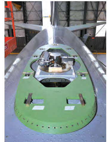
One of the Advanced Multiband Communications Antenna Systems (AMCAS) is ready to undergo flight testing to demonstrate the viability of using low-profile antennas on widebody aircraft to achieve multi-Mbps communications via military satellite communications.
