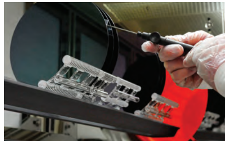
ABOVE, CLOCKWISE FROM TOP: A technician performs bright-light inspection of a 200 mm wafer prior to 3D bonding; chase view of one of the new 200 mm-wafer metal-deposition cluster tools; a 200 mm wafer being loaded into furnace.
