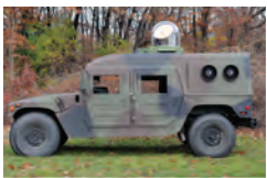
Jeffrey Hall of the Wideband Tactical Networking Group operates the Portable Army Communications-on-the-move Terminal Block 1 mobile SATCOM terminal that demonstrates the ability to have mobile communications that are robust to disruption by jamming or other attacks.
