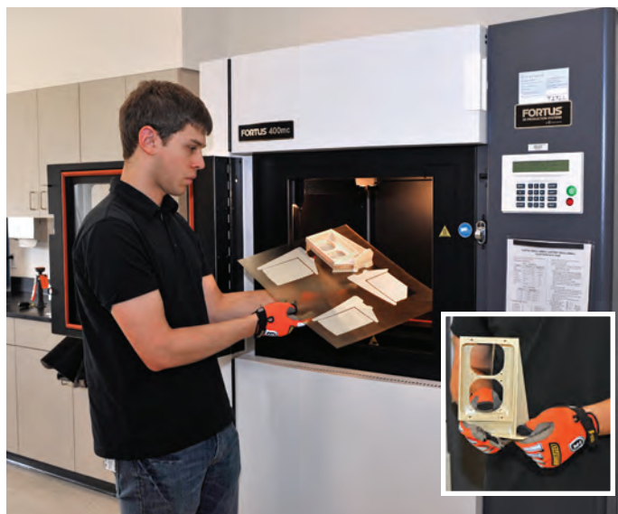
Michael Stern is shown building thermoplastic parts using a fused deposition modeling production system located in the Laboratory's new rapid prototyping facility. The system is used to rapidly produce parts and iterate designs, including fabrication of functional parts using advanced high-strength materials.
