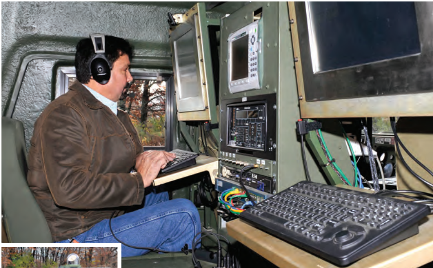
Jeffrey Hall of the Wideband Tactical Networking Group operates the Portable Army Communications-on-the-move Terminal Block 1 mobile SATCOM terminal that demonstrates the ability to have mobile communications that are robust to disruption by jamming or other attacks.
