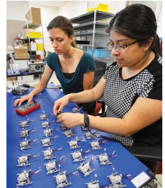
Mentored by Leslie Watkins (back), GEM fellow Marissa Garcia investigates small propeller motors in preparation for miniaturizing a camera payload for a micro-unmanned aerial vehicle platform.
