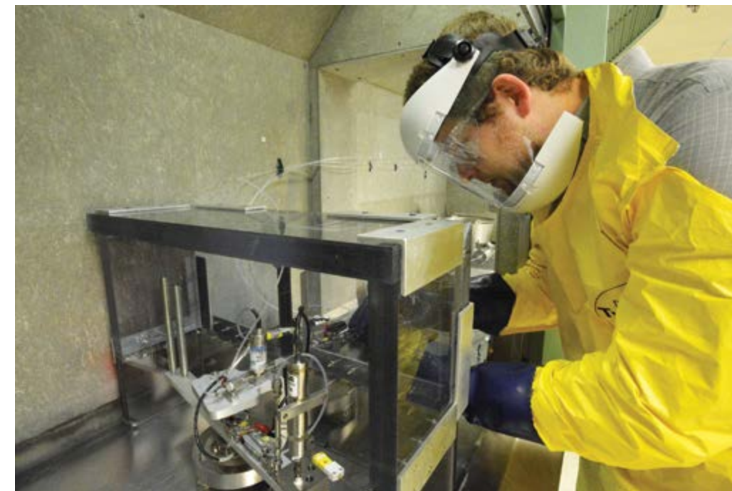
WPI student Orland Lamce (left), mentored at the Laboratory by Adam Shabshelowitz and Jesse Mills, prepares to test a small monopropellant rocket motor on a torsional thrust stand instrumented with pressure and temperature sensors to monitor the rocket motor's performance. The rocket motor is intended for use in nanosatellites or in similarly sized platforms.
