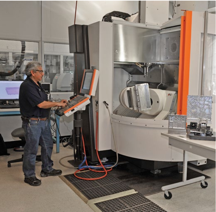
The five-axis machining equipment rapidly and efficiently produces components for prototype systems, resulting in savings in energy, manpower, and time.
