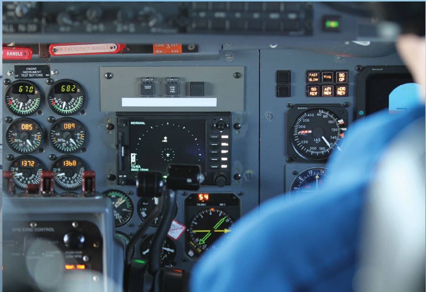
ACAS X (above) alerts pilots to nearby traffic and issues actions to avoid midair collision. The ACAS X flight-test team (left) gathers outside an experimental aircraft at the William J. Hughes Technical Center, the Federal Aviation Administration's national scientific test base and the primary facility supporting NextGen testing.
