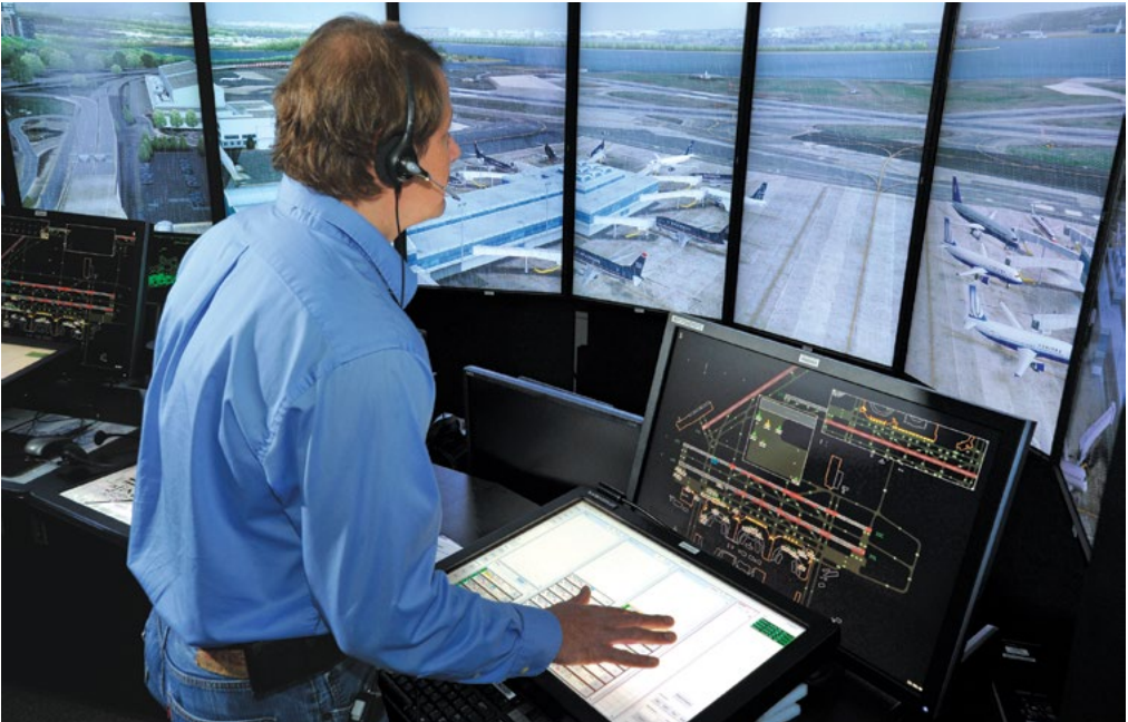
Lincoln Laboratory's air traffic control simulation facilities are used to design and evaluate new technologies for airport traffic management and integration of unmanned aircraft into civil airspace.
