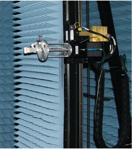
The near-field measurement range at the RF System Test Facility is used to characterize millimeter-wave imaging through common materials and to investigate sparse aperture sampling. Shown above are the near-field probes used for transmitting and receiving millimeter test signals.
