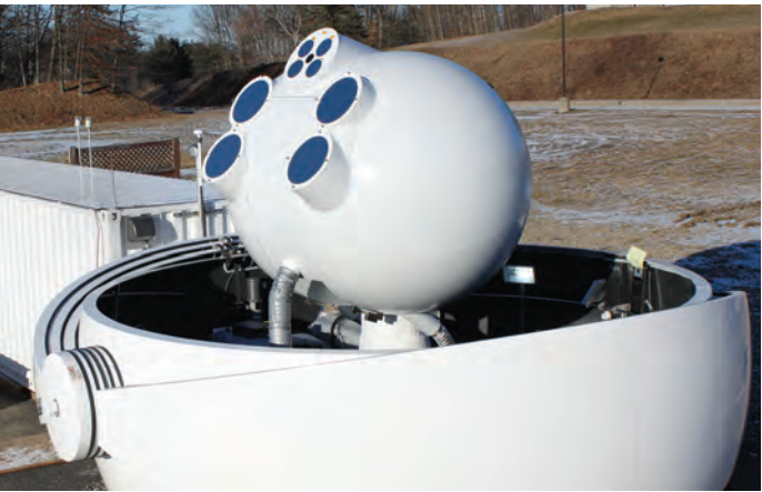
In this photo of the LLCD's transportable ground terminal, an array of four large downlink telescopes and an array of four small uplink telescopes are shown. The spherical enclosure keeps the system at a constant temperature, and the here-opened clamshell dome protects the system from the elements.
