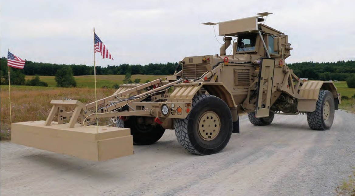
Lincoln Laboratory is developing new technology for conducting military missions with ground-penetrating radar. A prototype system is shown integrated on an Army Husky vehicle for combat evaluation.
