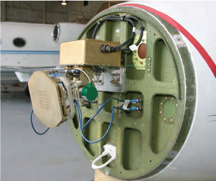
The gimbaled slotted planar array in the Gimbaled Airborne Test Radar test bed collects coherent range-Doppler measurements to demonstrate and evaluate the performance of advanced radar tracking and discrimination algorithms.
