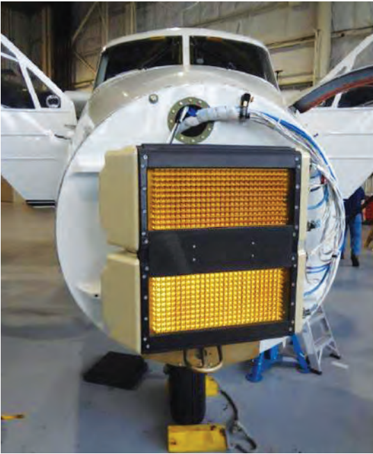
This Ku-band airborne sense-and-avoid radar, shown during installation on a Twin Otter aircraft, has separate transmit and receive apertures. The radar electronically performs a two-dimensional scan every 2 seconds and can search a 10 nmi area to locate a target as small as 10 dBsm.
