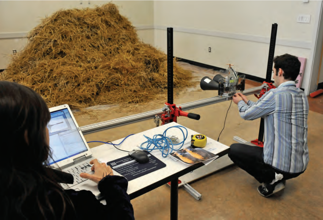
A new IAP course proffered a challenge: Find a Needle in a Haystack with 3D Imaging Radar. Participants set up an ultrawideband imaging radar that they used to image a haystack in which needles, skewered into Styrofoam balls, had been hidden. The onscreen image of the haystack (below) reveals the location of needles buried inside the hay. This two-day workshop built upon techniques covered in the other two radar-building IAP courses led by Lincoln Laboratory technical staff.
