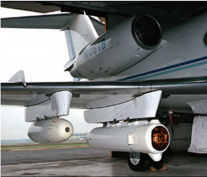
The dual-band, pod-mounted sensor developed for the Airborne Seeker Test Bed is used for airborne infrared imaging and data collection.
