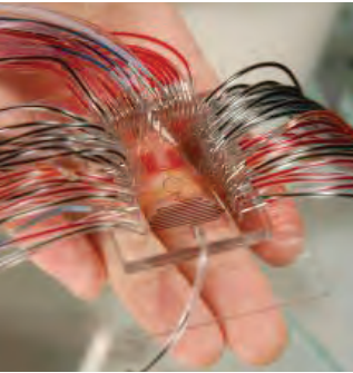
The Laboratory's biomedical sciences research includes enabling revolutionary, portable biomedical systems through the advancement of microfluidic devices. For example, the second-generation advanced Microfluidic Gene Assembler chips (above) now integrate 256 high-throughput microbiochemical reactors—a significant advancement beyond the first-generation devices (left) that prototyped single microbiochemical reactors.
