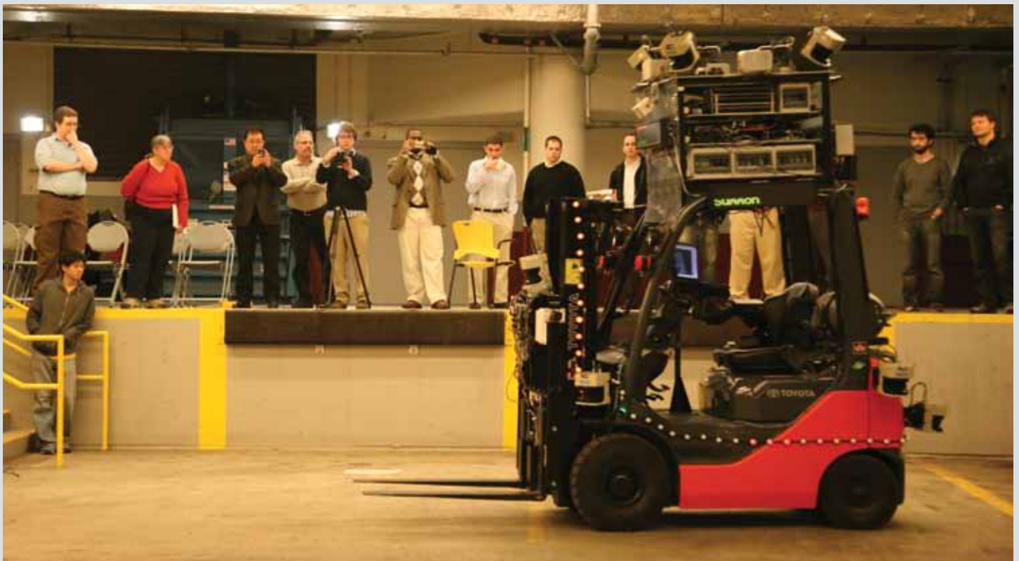
Lincoln Laboratory and MIT are testing a robotic forklift as part of a joint project for the U.S. Army. The forklift uses sensors developed for MIT's entry in the DARPA Urban Challenge. Eventually, the Army plans to employ the autonomous forklifts to haul materials onto robotic trucks.
