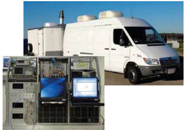
Lincoln Laboratory has developed a mobile electronics intelligence (ELINT) receiver test bed to detect and analyze RF signals in real time.
