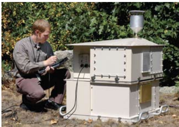
The Rapid Agent Aerosol Detection program is developing technology for high-performance, lightweight, integrated chemical and biological aerosol detection. Field trials have shown reduced false-positive rates and higher agent sensitivity over prior-generation detectors.
