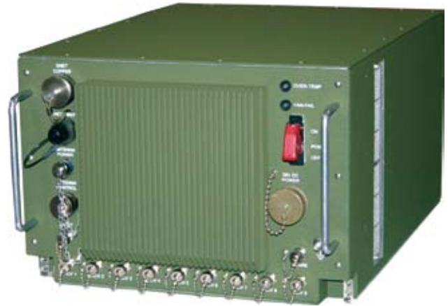
Lincoln Laboratory developed and successfully tested this multichannel signals intelligence receiver, which has enabled the Laboratory to rapidly innovate, develop, and test novel sensor capabilities for a variety of critical national problems. Key features include low noise figure, wide bandwidth, and direction-finding capability.
