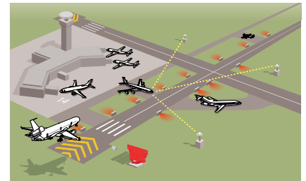
Runway Status Lights, under operational evaluation at Dallas/ Fort Worth International Airport, illuminate red to indicate that a runway is unsafe to enter or for departure. The lights operate automatically in response to real-time surveillance, providing improved situational awareness in the runway environment.
