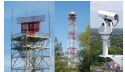
Existing ERSA sensors include FAA radars, elevated Sentinel radars, and EO/IR sensors.
