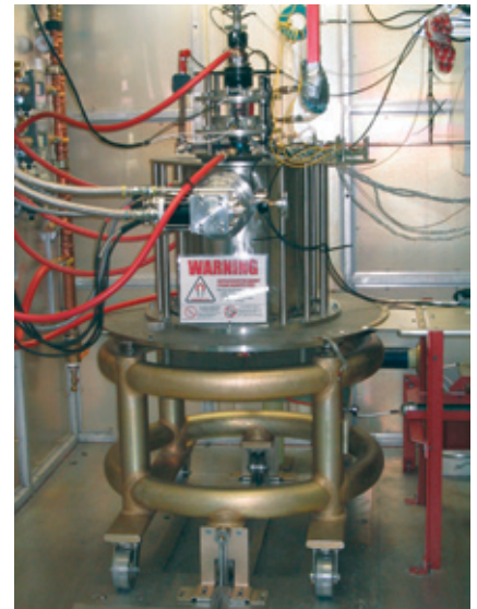
The low-power HUSIR transmitter uses a gyroTWT tube that covers 8 GHz bandwidth and produces 1,000 watts peak power.
