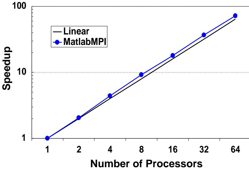
Figure 2: **Parallel Speedup.** Speed increase on the SGI Origin2000 of a parallel image filtering application as a function of the number of processors. Application shows “classic” super-linear performance (due to better cache usage) that results when a very large memory problem is broken into multiple small memory problems.
