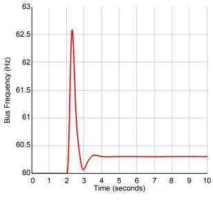
Figure 3 Genset Load Rejection Test
