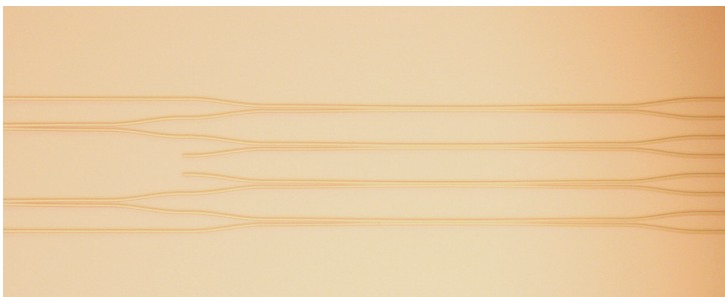
Optical microscope image of 3-dB adiabatic couplers in the active SiNx process.
