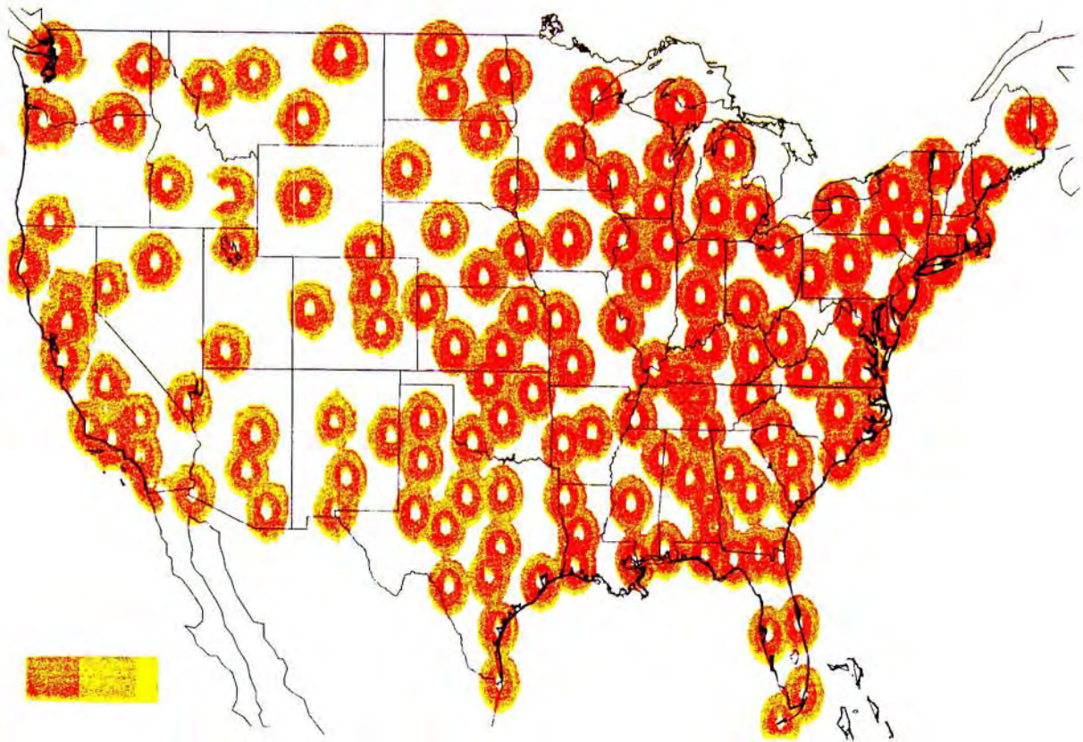
Figure 14 . NEXRAD three-dimensional coverage envelope as described in text.
