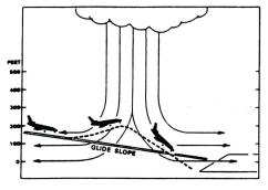
Fig. 1 Schematic drawing of an aircraft encounter with a microburst. Notice that the increased headwind lifts the plane above its intended glideslope while the increased tailwind causes the plane to fall below its intended glideslope.
