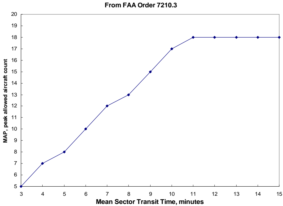
Figure 6. Monitor Alert Parameter density versus mean sector transit time.
