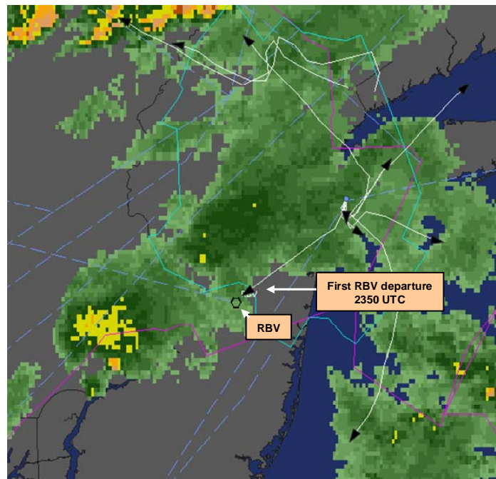
Figure A-1-2-2. Flight Explorer flight track and WSI composite reflectivity information at 0000 UTC on 06 July 2007. Black triangles denote airborne departures from JFK airport. The first of four JFK RBV departures to take advantage of the RAPT-derived early route reopening is approaching the departure fix at this time.
