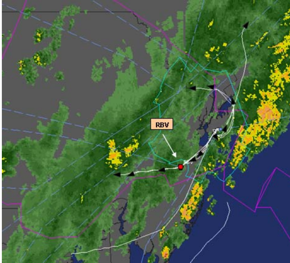
Figure A-1-6-2. Flight Explorer flight tracks and WSI composite reflectivity at 1840 UTC on 11 September 2007 showing JFK departures. At this time, all five JFK departures released via the RBV route between 1824-1837 UTC are airborne. ZNY used RAPT guidance (which predicted improving RBV conditions) to aggressively request five RBV departures at 1815 UTC.
